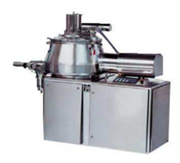
The powder raw material and adhesive in a cylinder are fully mixed at the bottom to become a humid soft material. Then it is cut by high-speed cutter and become uniform granules.
