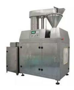
It is for compacting and granulating dry powder materials by using the crystal water contained (0.5-5%) in the dry powder itself. The machine is easy operation and cleaning, with compact structure, and high output and good fluidity. It is welcomed by users for its durability.
