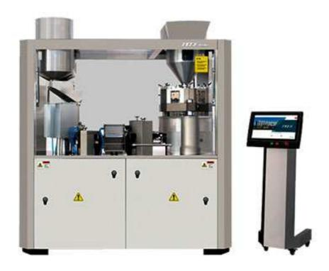
Siemens brand controller ensures the stability of electrical control system. The filling CAM acts directly on the filling mechanism, the tamping pressure is more stable, and the filling action is more accurate. Filling mechanism adopts profile-shaped multi-curved powder retaining structure, increasing flow support cone, making the powder surface in the powder filling ring more smooth, higher adaptability to powder, more accurate loading.
