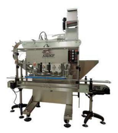
The fully-automatic, inline, six spindle SK6000X-BF6 Capper is designed for large cap applications. This machine features new 'Cap Correction Technology' to overcome cross-threading issues which are typical of large caps. It features an innovative belt feed system that eliminates vibratory bowls, overhead hopper loading and time-consuming changeovers on a range of flat caps.
