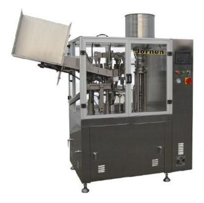
NF60A Automatic Tube Fillers are designed and engineered to produce outstanding quality and precision tube filling and sealing of plastic tubes with the output up to 60 tubes per minute. This machine is widely used in pharmaceutical, food, household chemical and cosmetic, etc., industries.
