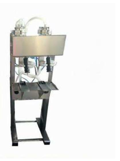
Perfume filling machine is used for filling floral water, perfume and other water-based materials. The machine adopts negative pressure and liquid surface type filling. It includes two kinds of specification such as four-head and six-head. Explosion-proof type products can be provided according to user requirements.
