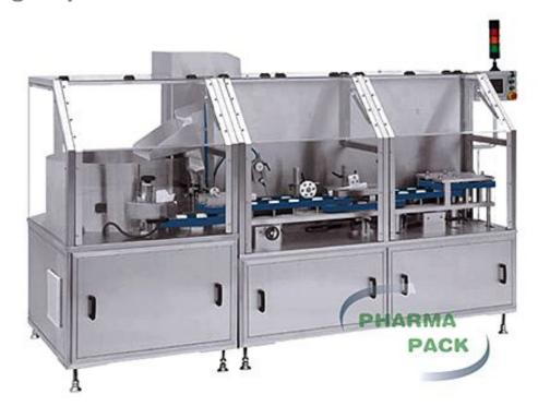
The unscrambler PU-25 is a reliable, high performance machine, designed in conformance with current and proposed GMPs. Having a small footprint due to compact design, it is effective in maintaining the integrity of a clean room environment. Few change parts are needed for different bottle sizes (only the presorter disc), and change parts are easy to dismantle and assemble, which ensures rapid size changeover and reduces the changeover downtime.
