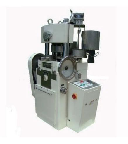
ZP13A/15A/17A/19A/21A rotary tablet press machine is a multi-functional rotary tablet press. It has a wide range of applications. This rotary tableting machine can be used for making watercolor tablet, disinfection tablet, camphor tablet, and so on. It can not only be applied in pharmaceutical, medicine, pill and foodstuff industries but also used in the chemical, ceramic, electronic and battery industries.
