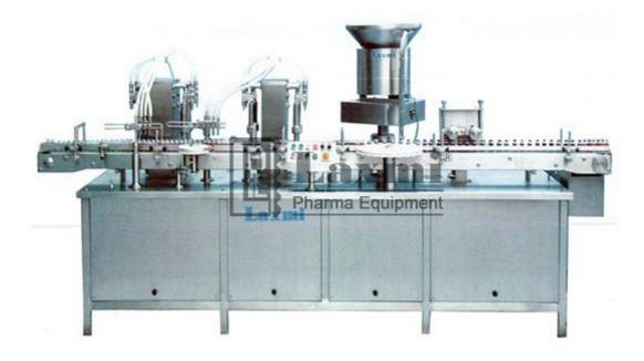
Laxmi Pharma Equipment offers compact automatic volumetric eight head vial liquid filling & rubbers stoppering machine mode: LVFS – 200R. The machine consist of turntables, S.S. slat conveyor belt, eccentric pre-gassing, filling & post –gassing S.S. -316 nozzles precision built S.S. – 316 Syringes, silicon rubber tubing's, easy – reach compact panel etc. Due to its minimum distance between filling and stoppering, the risk of contamination is reduced.
