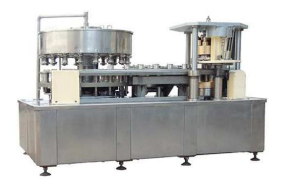
This combined machine is used for filling and capping of beer and other carbonated drinks. It adopts the most advanced mechanical, electrical, pneumatic control technique in the world. It has such advantages as stable filling, fast speed, control of liquid surface, reliable sealing, frequency modulation speed adjustment. We can install remote control system according to requirements of customer, it is priority and ideal facility for medium-size beer plant and beverage plant.
