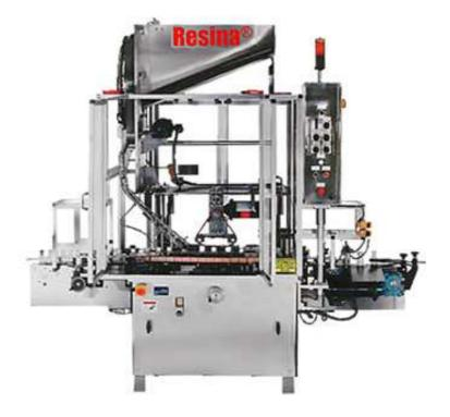
The NRF Fitment Applicator is designed to take fitments or "shaker tops" orient them, and place them in a container. Though mainly by customers in the spice industry, this machine is very versatile and has many applications. It comes equipped with our H-26 cap hopper / sorter which is the best on the market. Also, NEMA 4 control panel, 8' of conveyor, and complete safety guards are all standard.
