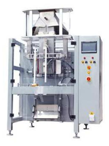
Vertical auto packaging machines is suitable for packaging various kinds of leavened food, candies, peanuts, seeds and such materials in grain or piece as well as powder like milk powder, washing powder, starch, etc.
