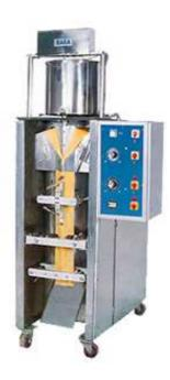
For Packaging of liquid such as Mineral Water, Milk, Soft Drinks, Lassi and Country Liquor. The system does not require any compressor or compressed air.
