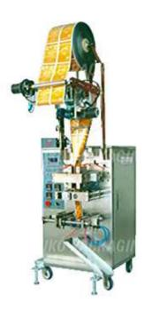
The MK-212 is a Fully pneumatic vertical form fill seal packaging machine designed to package free flowing liquid products. This Fully automatic vertical VFFS packaging machine uses volumetric piston filler system to produce center sealed, 3 side sealed and 4 side sealed pouches / bags.
