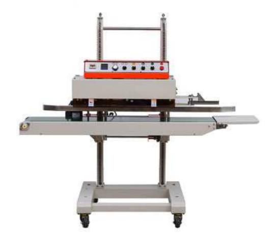
The series sealer is in the function on continuous carrying, sealing and printing in one operation. The machine can be made horizontally, vertically or with stand feet. It adopts electronic constant temperature mechanism and stepless speed regulating transmission motor. It can seal plastic film in various kinds of materials.
