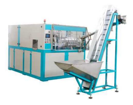
The conveyor put the preform from the barrel to the entire machine, then the preform is automatic arranged in order to feeding in a single way Adopt FESTO rodless cylinder to divide into blank movement and positioning. The clipper picks preforms is place them on the transfer system. The way will avoid preforms jamming or wasting preforms.
