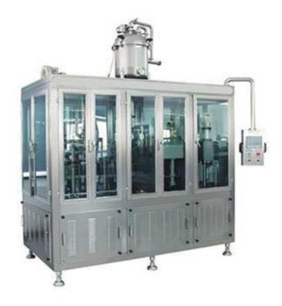
This equipment is used for packaging liquid drinks including fresh milk, fruit juice, acid milk product, etc. The production capacity is 1000box/h. The pack is 250-1000ml standard gable paper box. The main characteristic of this equipment is: high adaptability, little investment. The machine is of convenient operation and stable function, which is the best choice of drinks industry for high grade package improving of the image and enlarging the sales market.
