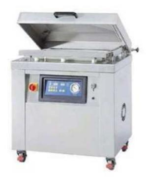
The packaged products can be prevented from oxidation, going mould, insects or getting damp, thus can be kept fresh after closing the lid, the machine can automatically run through the full cycle of installed functions, including vacuum extraction, insert gas flushing (optional), sealing, printing, cooling and exhaust. The packaged products can be prevented from oxidation, going mould, insects or getting damp, thus can be kept fresh in a prolonged storage time.
