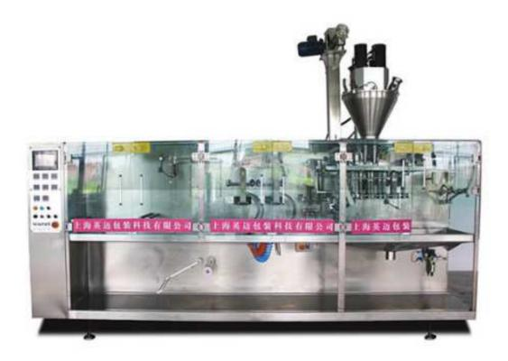
This machine is made with the combine of technology and innovation, it has stainless steel frame and it fills 100gr. In optimum conditions it can reach 90 packs per minute. For all of the electronic and pneumatic parts used world-known brands. And also this machine has half cut unit.
