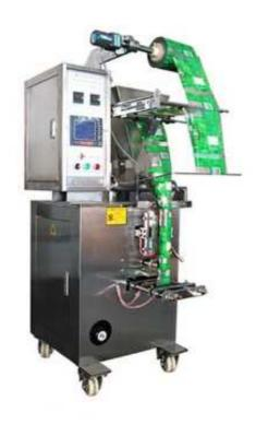
This machine is suitable for small sachet packing or powder material which with bad fluidity like milk tea, milk powder, soya flour etc.
