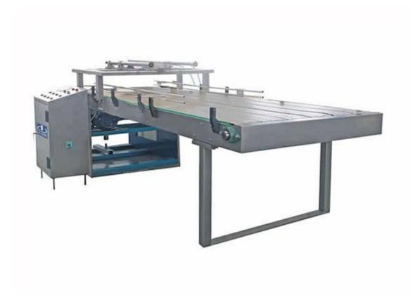
Orientator bottles DSP100 / 500 is used to promote and organize bottles for infusion solution in the cards for sterilization after the end of the closing procedure. The equipment consists of a section of the promotion of bottles and bottle storage section; due to the high degree of automation, it is able to reliably perform all procedures.
