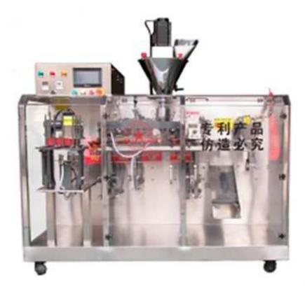
This premade zipper pouch filling sealing machine is a low cost mini doypack powder packing machine. It is for picking filling sealing premade zip lock bags, spout doy packs fully automatically, etc.
