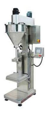
The semi automatic weighing and filling machine is mainly designed for ultra-fine powder and high-precision packaging requirements that are easy to dust. It performs two-speed filling, metering and lifting according to the signal given by the weight sensor mounted under the container. It is suitable for packaging milk powder, additives, Toner, dry powder for fire extinguishers, other ultrafine powders, and powders with high precision packaging requirements.
