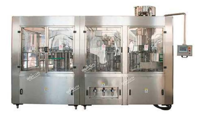
This High Speed Carbonated Beverage Filling Packing Machine is mainly used for carbonated beverage filling capping. The machine is 3 in 1 monoblack composed of washing, filling, capping in one unit. The rinsing head adopts overturning device, and filling system is gravity filling type, it's more stable and reliable.
