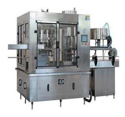
This production line is fully automatic. It is mainly used for washing, filling and sealing of three piece can style pop-top cans made of tinplate.
