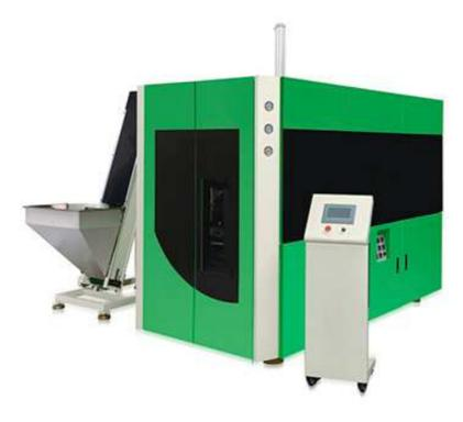
**WBB-4S** Single Servo Motor Bottle Moulding Machine is a 4 cavity automatic Bottle Blowing Machine, which output is about 4000BPH. max. blow bottles 2L. It is used to blow bottles from PET preforms which can be bought from the market directly, or produced by our injection molding machine and PET Preform Mould. We will design the bottle shape basing on clients 'requirement before making bottle mould. Also suggest the preform weight basing on bottle type and design.
