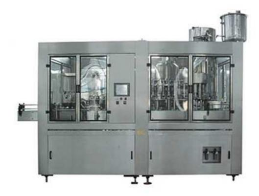
The design is scientific and reasonable. Good appearance, easy operation and convenient maintenance. The machine adopts block bottle-neck hanging work state design, and adopt filling valve rise-drop designing. It's designed for 95°C hereinafter hot filling technology demand. It adopts person-machine interface touch-screen, PLC, transducer etc advanced control technology. Material contact with drink is SUS304 stainless steel.
