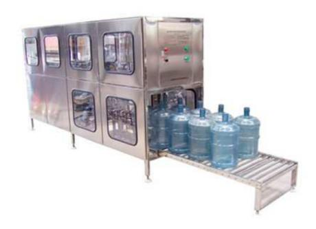
This machine is a washing-filling-capping integrated machine, which is mainly used for 5 Gallon bottled water filling process. It is designed for shortening the contact time between drink material and outside, so as to improve the sanitation condition of the water product and increase the economy benefit.
