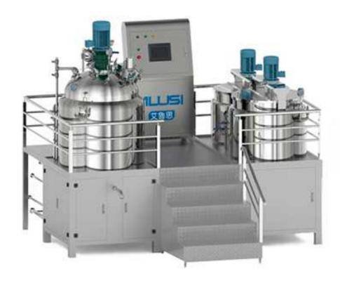
Fixed Vacuum Mixing Machine is mainly composed of water pot, oil pot, emulsifying pot, vacuum system, PLC control system (electric is optional), operation platform, etc.
