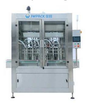
CCG5000-6D type intelligent high viscosity filling machine is suitable for the packaging of various water agent, emulsion, oil suspension, suspension agent and high viscosity materials. The whole machine is inline structure, using servo motor drive and volume measurement and filling principle to realize the high precision of filling dose. PLC control, touch human-machine interface, convenient operation.
