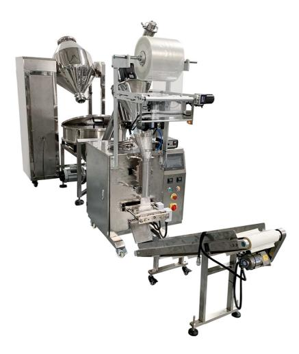
The powder mixing and packaging machinery can pack the Max. powder about 250gr of pillow bag.
