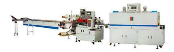
The machine is suitable for assembly shrink packaging of the products such as cup-shaped and box-shaped products like cup noodle, and for group shrink packaging beverage bottles, books, batteries, soaps, daily necessities, machine parts, etc.
