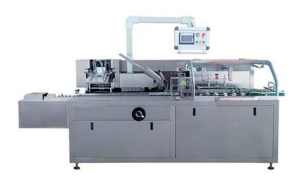
PZH-100A Automatic cartoning machine is a high-performance product that integrates electromechanical, gas, and light-based on foreign advanced equipment introduction. It meets GMP requirements. The machine is a continuous operation, automatic box opening, leaflets automatic folding(1-4 folds), printing batch number sealing detection and other functions (can also be equipped with hot melt adhesive device), the highest speed up to 80-90 boxes/min.
