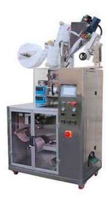
This is our full automatic drip coffee bag packing machine, it makes drip coffee bag (with paper hanger) with outer envelop automatically, the machine weighing by screw auger, it controlled by PLC, and all the parameter setting like tea bag shape changing can be finished on the color touch screen. There is vacuum feeding machine, date printer optional.
