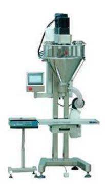
LG-BLG series semi-auto screw filling machine is designed according to the standards of Chinese National GMP. Filling, weighing can be finished automatically. The machine is suitable for packing powdery products such as milk powder, rice powder, white sugar, coffee, monosodium, solid beverage, dextrose, solid medicament, etc.
