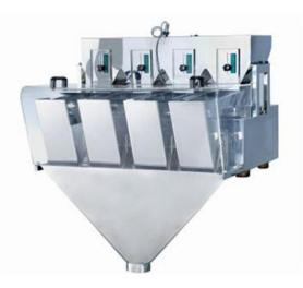
The four head linear weigher is equipped with four heads for the synchronous weighing of 4 different materials and each hopper features a weighing range of 20-2000g. By pairing with packaging machines, this linear weigher is capable of packaging mixed materials with four components. It is simple to change products and target weight. Due to quick changeover, the four head linear weigher is ideal for the packaging of uniform granule mixtures with different weights and components.
