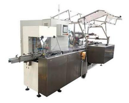
The machine is mainly used in the food, medicine, soap and cosmetics packing etc. It is designed with hot glue sealing or tucker type sealing systems. Chinese/English touch screen is easy to operate and do the parameters setting. PLC is used for accurate control, fast response, and high reliability. Hot glue temperature is auto controlled for easy adjustments.
