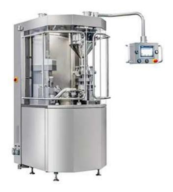
The SFK-700 is designed to produce 42000 capsules per hour. The device is suitable for low and medium batch production and frequent product changes. The equipment complies with GMP standards and can quickly complete mold conversion and implement equipment cleaning.
