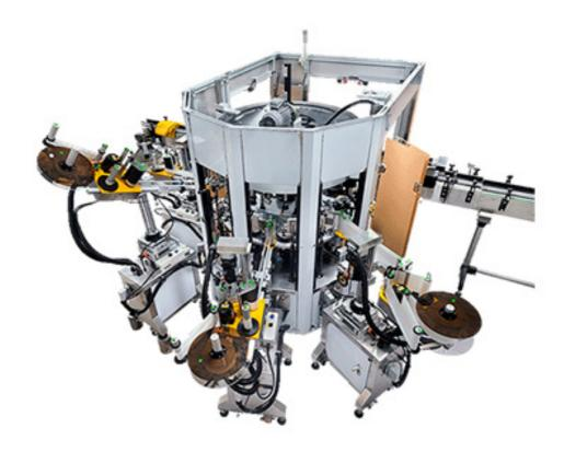
Suitable for applying more than three labels on the same bottle and can complete various labeling types such as side label, back label, neck label, small label, etc. which is suitable for labeling different bottle types on the same machine (such as whisky, sake, sauces, seasonings), and one machine can meet various labeling demands. Solve the shortcomings of traditional models that cannot be used for multiple purposes.
