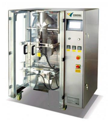
This machine is applicable for packing granulated, short stripped and powdered stripped products, such as puffed food, shrimp, peanuts, popcorn, oat cereals, melon seed, frozen fruit, sugar, edible salt and washing powder, ect.
