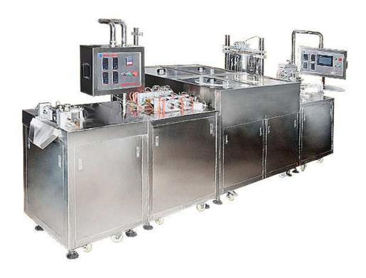
The machine is driven by electricity, gas, controlled by PLC operation, with PVC/PE film as packaging material automatic production suppositories product equipment Molding of heat generated by the temperature elements and maintain, molding pressure by multiple groups will be compressed air cylinder converting mechanical energy form.
