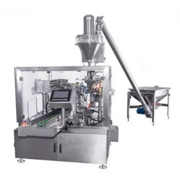
This series auger filling machine is designed mainly for fine powder which easily to spout dust & high-accuracy packing requirement. Based on the feedback given by below weight sensor, then machine complete double speed filling, measuring, up-down work etc, it is suitable for additive, carbon powder, fire extinguisher powder, other fine powder which needs high packing accuracy.
