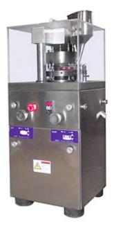
The machine is a single-press type, continuous automatic tablet press for pressing granular raw materials into tablets. It is used for small-scale production.
