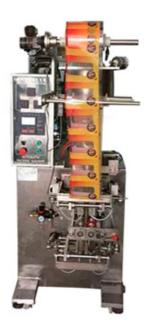
This coffee powder sachet packing machine adopts correcting system controlled by microcomputer, owing to a response signal is handle and pass through microcomputer. it can accomplish whole set to synchronization, sack length, position fixing, voluntarily follow the tracks of light-mark and voluntarily diagnose trouble and show to screen.
