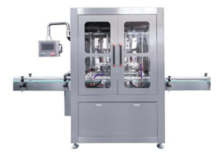
The NP-TVF Automatic Tracking Piston Filling machine is the new generation piston filler. The update is the control technology, not the volumetric dosing system. it adapts with emotion controller, servo motor driven the moving of the pistons and filling heads. It is non stop and continuous working. The machine is working more efficient and intelligence, multi-axis high-precision synchronization controlling working.
