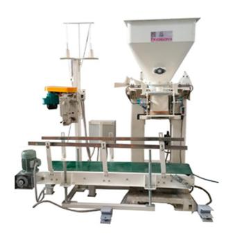
Open-mouth bagging machines' represent a mainstay of modern industrial packaging solutions and have no equal in terms of efficiency and precision. These are the cornerstones of packing operations across different sectors such as agriculture, food, pharmaceuticals, etc. Open-mouth bagging machines simplify the process of filling and sealing bags having varying contents like granules, powders, or aggregates.
