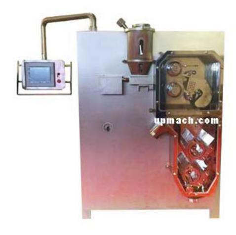
Roller Compactor, known as Dry granulator, is new self-developed equipment which is integration of the extrusion, pulverizing and granulating, also belongs to new equipment with function of energy-save and environment protection.
