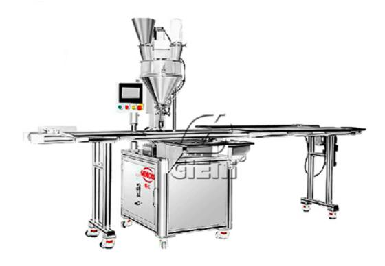
This production line is designed to filling loose powder into Jars, like nail powder, eyeshadow, face powder, talcum powder, or other powders. It comes with auto filling and weight checker, east to operate and clean.
