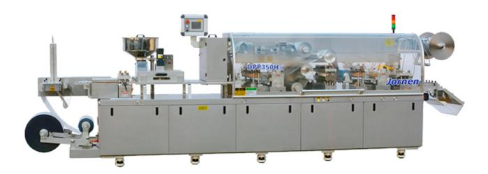
This Blister Packaging Machine adds one tropical alu forming station and a second sealing station to allow the plastic thermoforming blister package to be sealed with formed tropical alu again.
