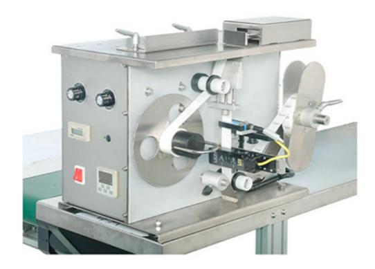
This machine suitable for corner labeling for various carton box products.
